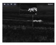
indicates the center position of the reticle. At this time, press the UP button to switch the PIP magnification. The original image will maintain a x1 magnification.
