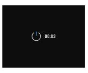
Tips: If you release the POWER button within 3 seconds, the shutdown process will stop and it will return to the main interface.
